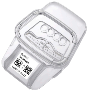
EmbryoSlide+ culture dish For embryo culture in the EmbryoScope+ and for the Embryoscope 8 instrument. Each EmbryoSlide+ culture dish contains 16 microwells for incubation of up to 16 embryos.
