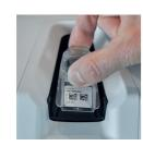
Discrete loading area means incubation conditions are virtually unaltered when dishes are added or removed.
