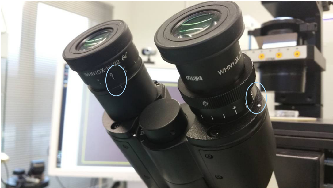
Fig. 56: Diopter adjustment (example: Olympus inverted microscopes)
