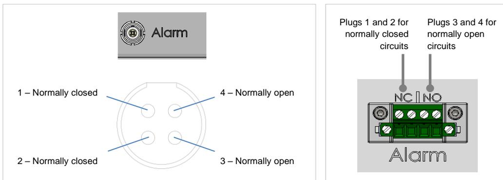
The EmbryoScope+ incubator supports two types of circuits: normally closed or normally open. The connected external alarm system should match the chosen circuit.
