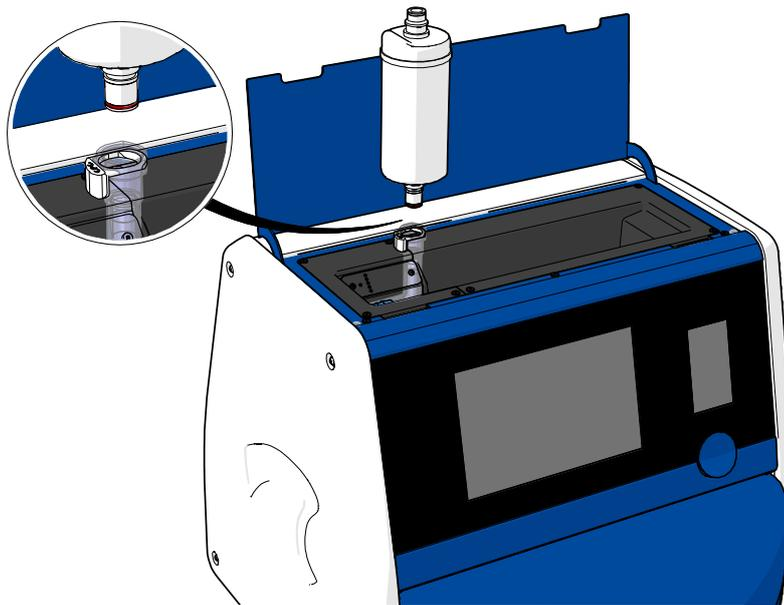
6. Insert a new VOC HEPA filter by reversing the removal procedure:
