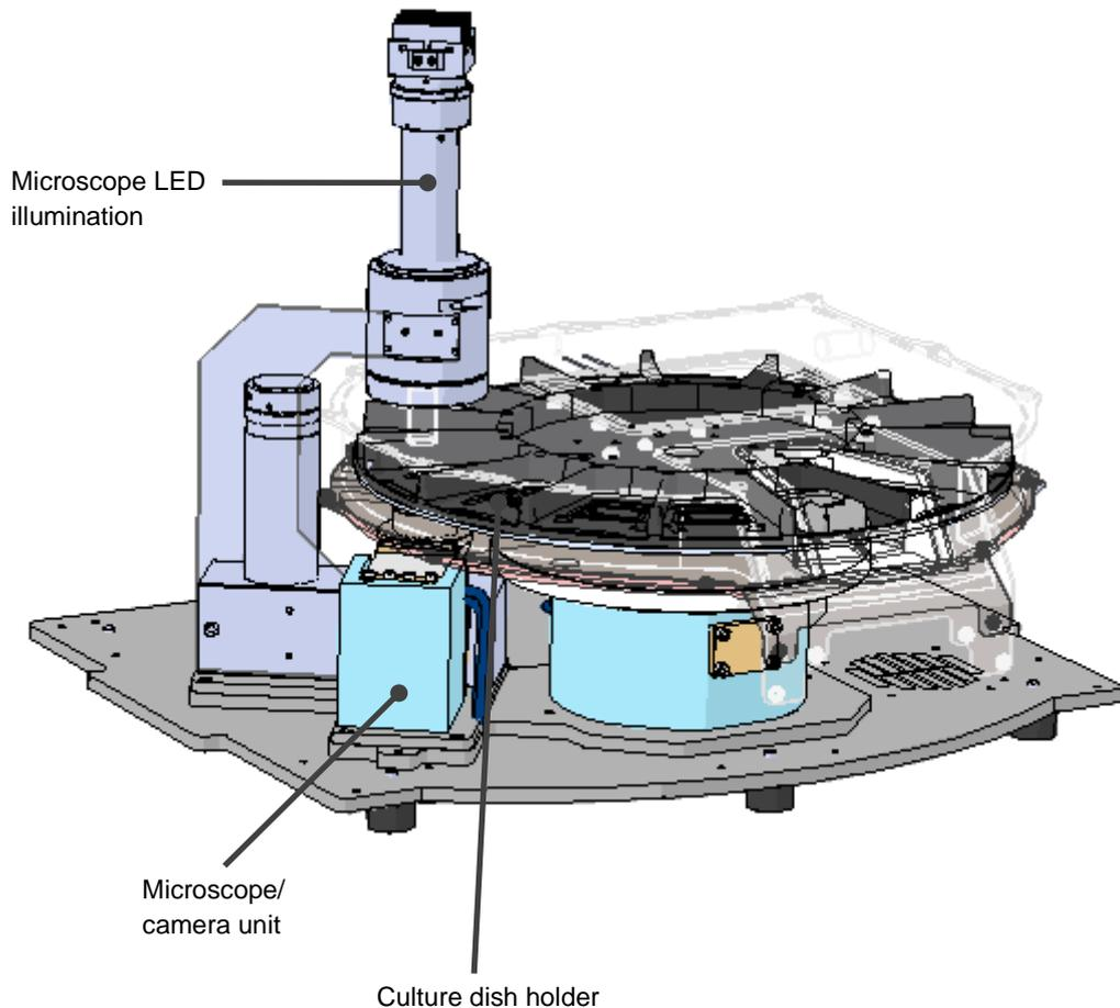
The culture dishes are placed on the culture dish holder in the EmbryoScope+ incubator. The culture dish holder is a sandwich construction controlled by a thermostat. The holder provides direct heat transfer to the culture dishes and automatically moves the culture dishes from load position to camera position during time-lapse imaging.
