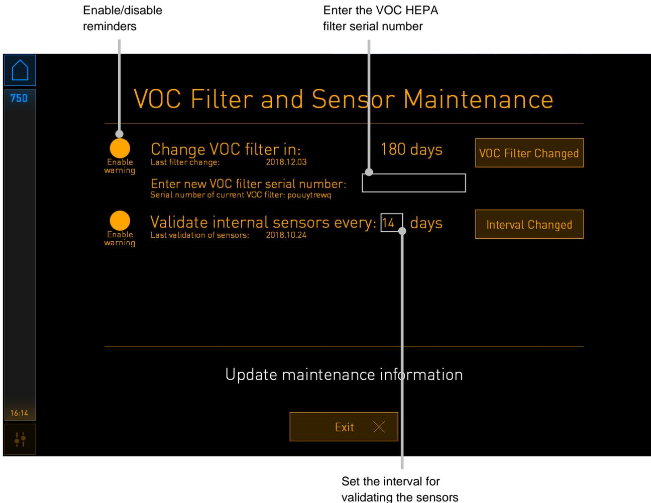
The interval for changing the VOC HEPA filter is 180 days. When the VOC HEPA filter is changed, you will be prompted to enter the serial number of the new VOC HEPA filter. Enter the serial number, and press the **VOC Filter Changed** button.
