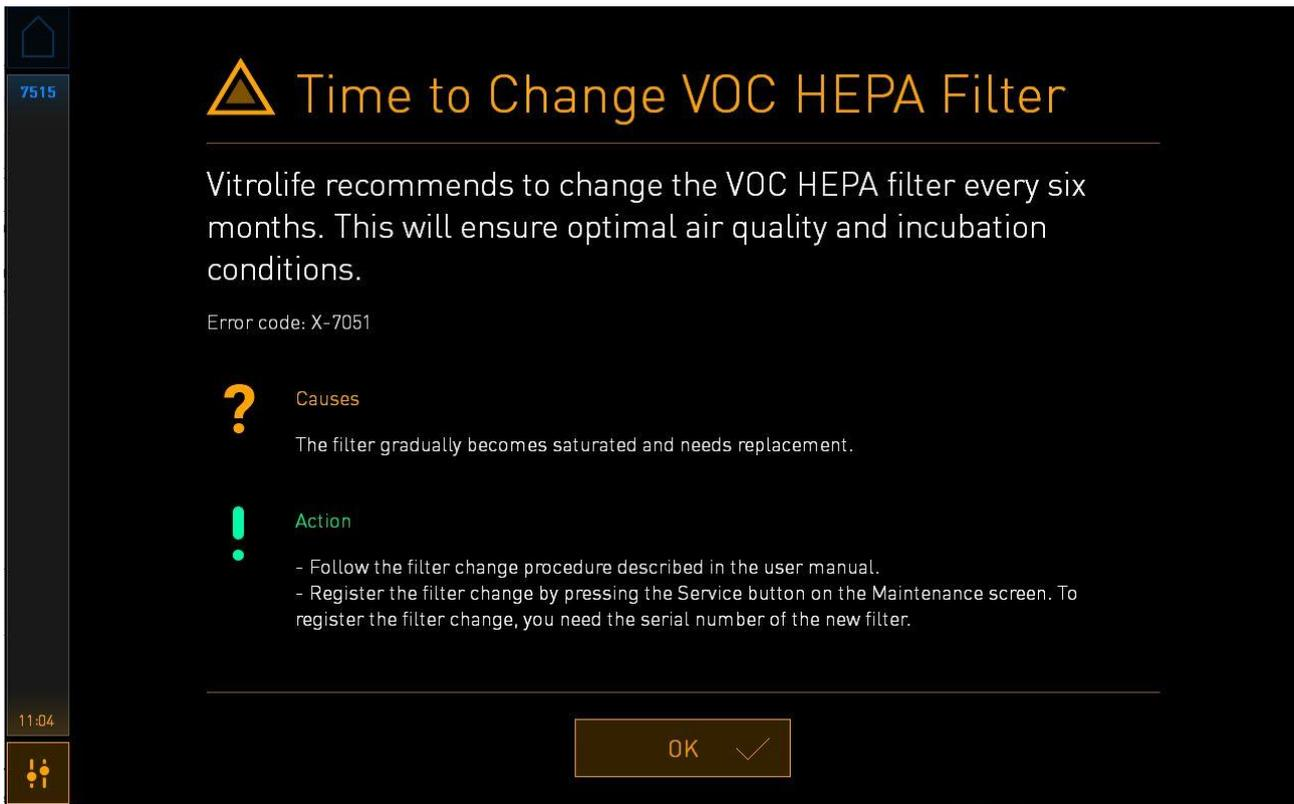
If you press **OK**, the warning will disappear and remain hidden for three days. If you do not change the VOC HEPA filter within this period, the warning will reappear. You can press **OK** as many times as you like, but the warning will reappear every three days until the filter is changed.
