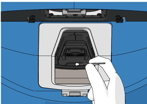
9. Manually rotate the culture dish holder to the next position until all contaminated positions have been cleaned as described in step 8.
