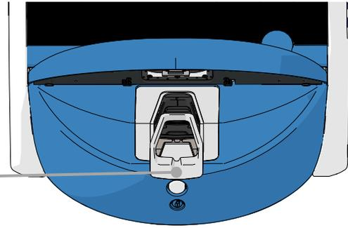
4. Manually rotate the culture dish holder clockwise until a culture dish appears. Then remove the culture dish and place it in another incubator.
