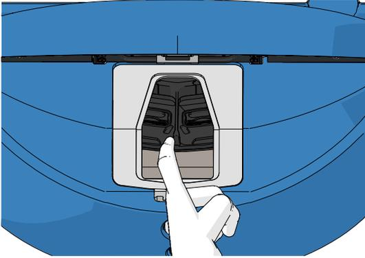
10. Clean the load area frame: Apply clean, distilled water to lint-free tissue wipes and wipe the load area frame. Repeat until the wipes are no longer discoloured.
