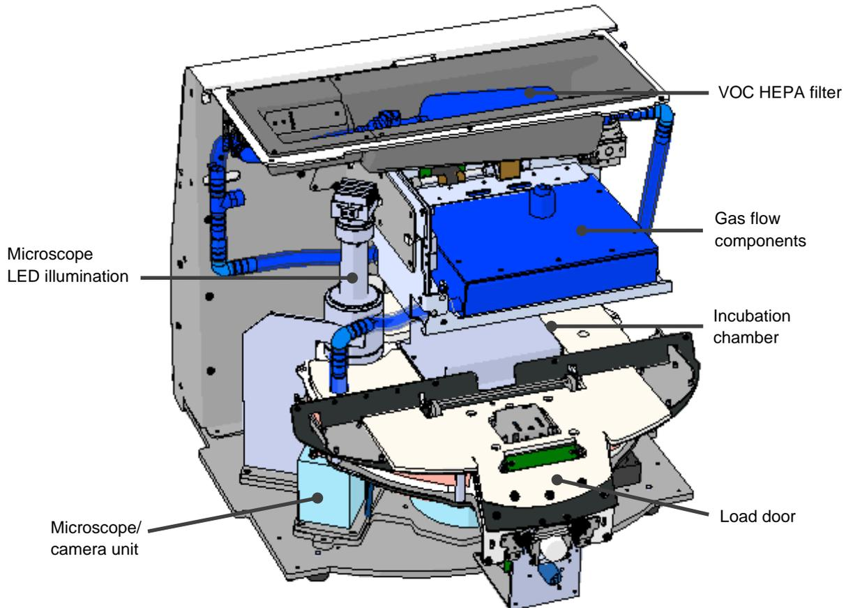
The blue components in the above illustration represent the gas and temperature system of the incubator. These components maintain the desired gas concentrations inside the incubation chamber. The gas is circulated through a VOC HEPA filter before entering the incubation chamber. The same system also controls the temperature conditions inside the incubation chamber.
