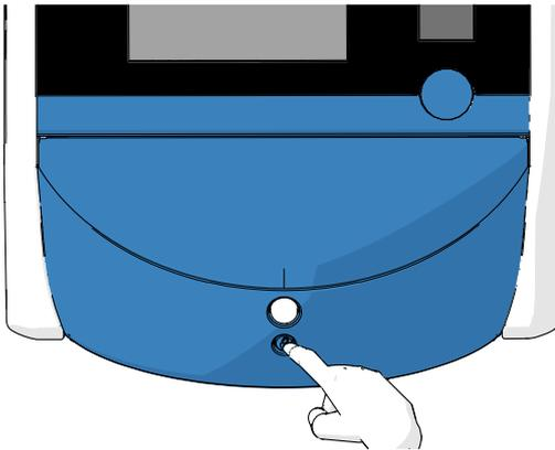
5. Open the load door to the incubation chamber by pressing the white load door open button.
