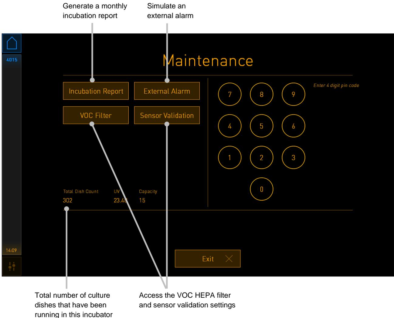
The pin code on the right side of the screen provides access to advanced maintenance functions to be carried out in collaboration with Vitrolife personnel. Vitrolife will issue a pin code if this is relevant.
