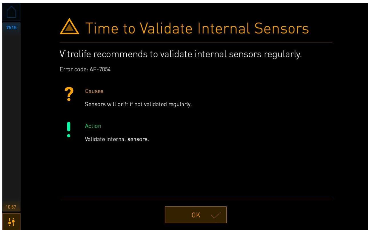
If you press **OK**, the warning will disappear and remain hidden for three days. If you do not validate the sensors within this period, the warning will reappear. You can press **OK** as many times as you like, but the warning will reappear every three days until the sensors are validated.
