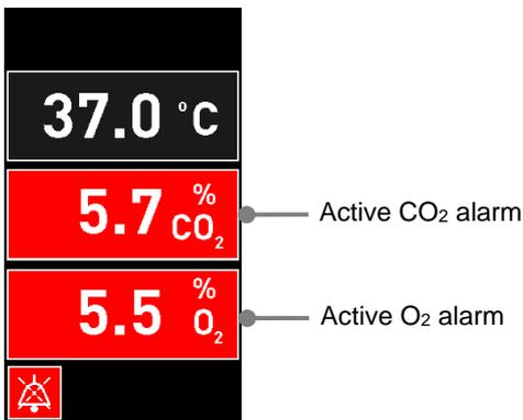
It will not be possible to return to the default incubator home screen, change set points or calibrate the internal sensors until all active alarms have been resolved (displayed in orange colour) and reset.
