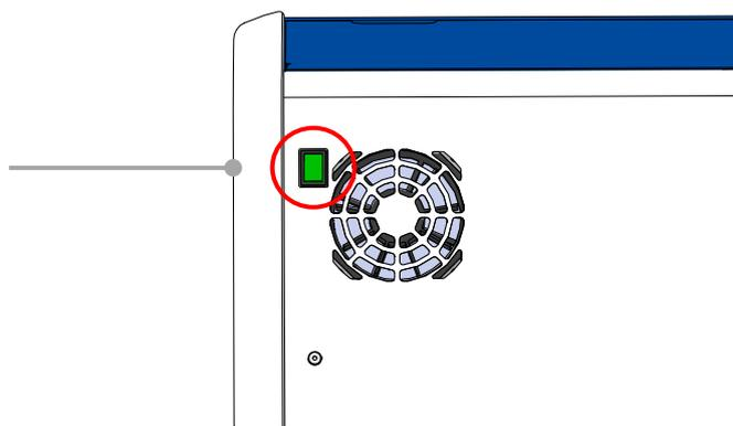
2. Press the emergency unlock button at the front to unlock the load door. Then press the white load door open button.
