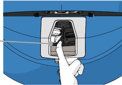
5. Remove the rest of the culture dishes by rotating the culture dish holder again and removing the next dish. Repeat as many times as possible until you reach a hard stop. Then rotate the holder counter-clockwise as many times as possible until you reach a hard stop.
