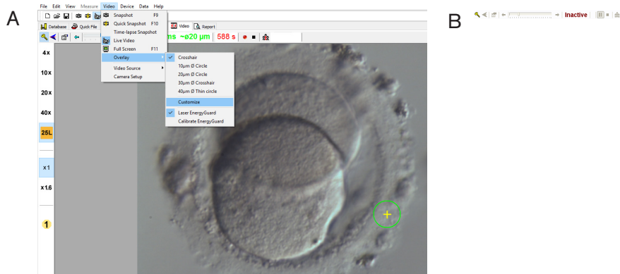
Fig. 54: XY positioning of the crosshair. A: dropdown menu. B: Video Overlay window for moving the crosshair position.
