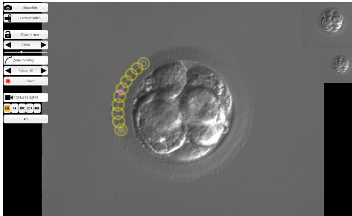
Fig. 25: NaviLase operational mode for drilling holes along a predefined curved line
